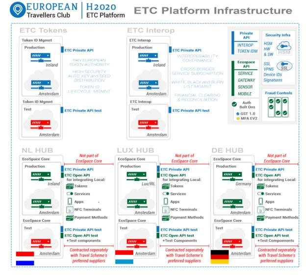
The ETC Platform, consists of a Token ID Mgmnt Module to distribute unique side tokens to Legacy Travel Cards, an Interoperability Hub to allow Travel Scheme Travellers to travel in between participating Travel Schemes based upon Inter-Scheme travel agreements and a series of Travel Scheme Hubs to allow each Travel Scheme to attach their preferred Cloud Ticketing and Cloud Payment services locally.
